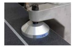
The latest technology of air bearings is incorporated into the design to sense the slightest movement.
