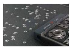
EROWA workholding systems can be mounted directly on the granite slab thanks to their standard hole pattern.
