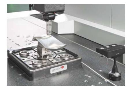
During "normal measuring", only individual points are measured. With scanning, a large amount of data is recorded. This generates much more detailed information about the form and shape of the workpiece.
