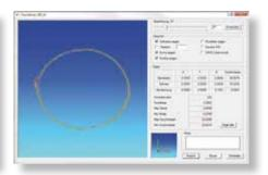
Both the number of measured points and the results of this roundness measurement using scanning are clearly displayed.
