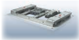
Multiple-part palletizing increases the autonomy of the machine. Makes use of the unmanned shift.
