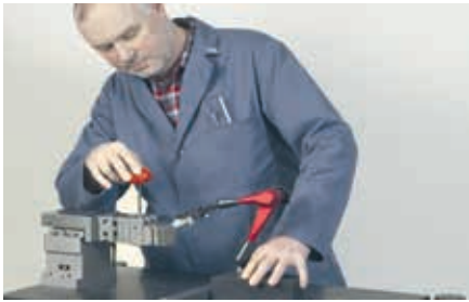
Determining starting borehole coordinates, establishing the spatial location of workpieces, and performing quick intermediate checks.
