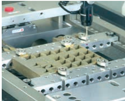
Accurate presetting of workpieces facilitates subsequent work.
