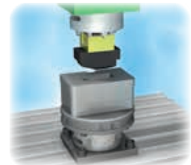
15 Put workpiece and electrode on EDM then start EDM-ing
