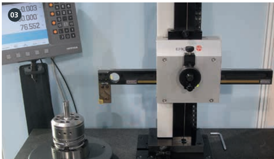
The pallet is clamped pneumatically on the alignment device – Repeatability < 0.002 mm.
