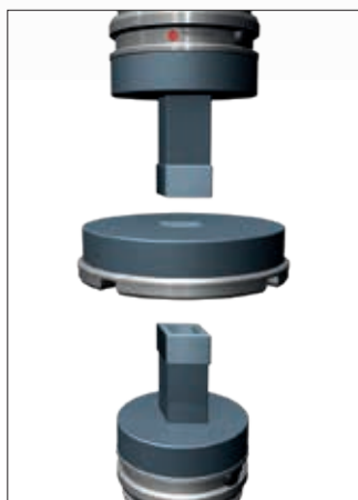
Insert and clamp new dies and punches.
