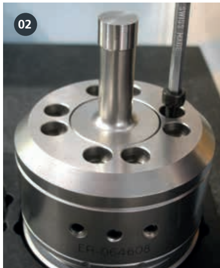
The punch can thus be mounted and clamped in the adaptation pallet.
